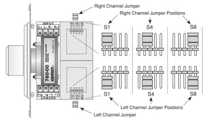
Fig. 2 Jumper Placement For Impedance Matching
